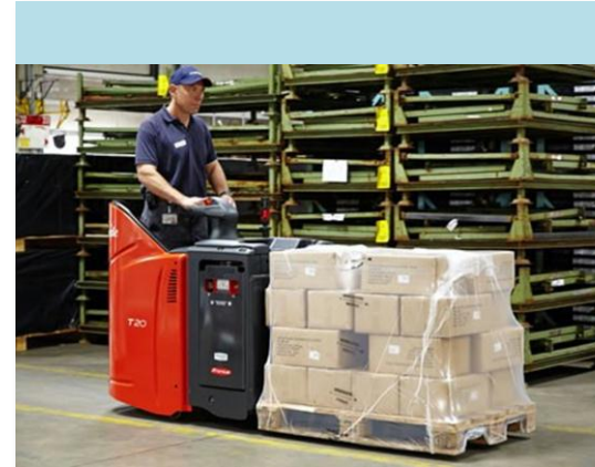
Linde T20 pallet trucks with fuel cell hybrid drive operating at DB Schenker's Linz, Austria facility
