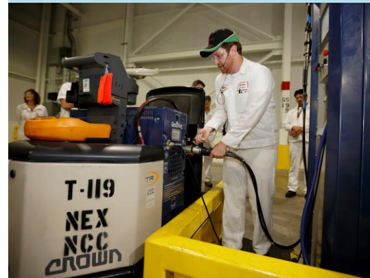
Refueling with hydrogen at Honda's Marysville, Ohio site
