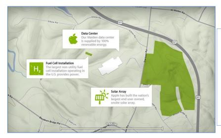
Apple's Maiden, North Carolina data center includes 10 MW of fuel cells and 20 MW of solar power. Note the relative size differential between the fuel cell installation and solar array.
